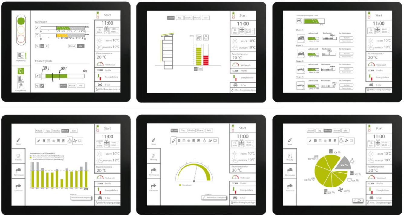
Figure 4: Sample Pages User Interface: Home Page, Energy Balance, E-Mobility, Electricity Consumption (Month, Real-Time and Comparison of different Consumers within the household); Source: Unit of Design & Energy Efficient Building, TU Darmstadt
